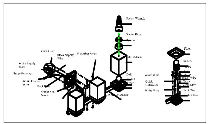
Line art shown may not exactly match the fixture enclosed. However, the installations do apply to this fixture. ITEM NO:1916-1S,1916-2V/3V/4V/5V
