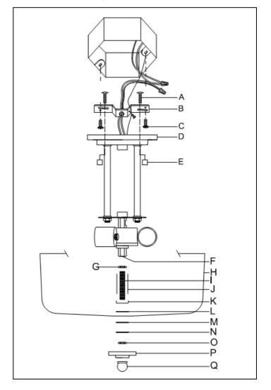
Line art shown may not exactly match the fixture enclosed. However, the installations do apply to this fixture. ITEM NO:414SF 434-SF-BN
